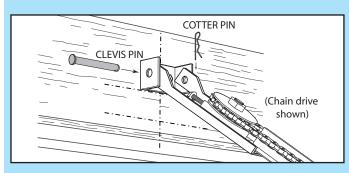
FIG. 2-5 Rail mounting to header bracket.
